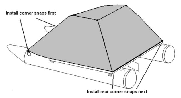
You will need a power screwdriver with a #2 Phillips head bit and some chalk. You will need to remove canopy (or lay the canopy completely down on the rear deck) as the mooring cover will not fit over the canopy when it is in the upright position. We recommend inside storage for the canopy top if you are storing it for the winter. You will also need to remove the table unless you have a cover that accommodates the table. Note: Do not over-tighten screws!
